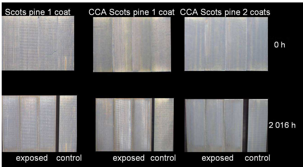
Figure 8 : Appearance of the Scots pine samples coated with the stain 3C before and after EN927-6 test
